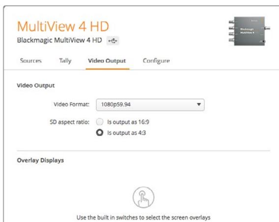
The 'video output' tab for Blackmagic MultiView 4 HD lets you set the output HD resolution and frame rate, plus set it to interlaced or progressive scan
