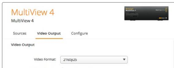
The 'video output' tab for Blackmagic MultiView 4 contains a dropdown list of video format options that covers both resolution and frame rate
