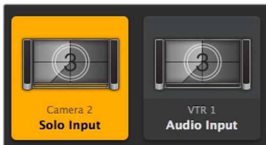
The "solo input" and "audio input" pushbuttons allow you to change these settings using Videohub Control
